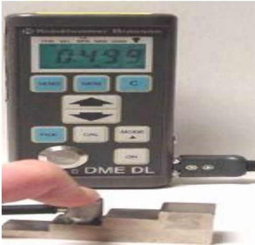
Figure. 2 Calibration of ultrasonic thickness gauge.
