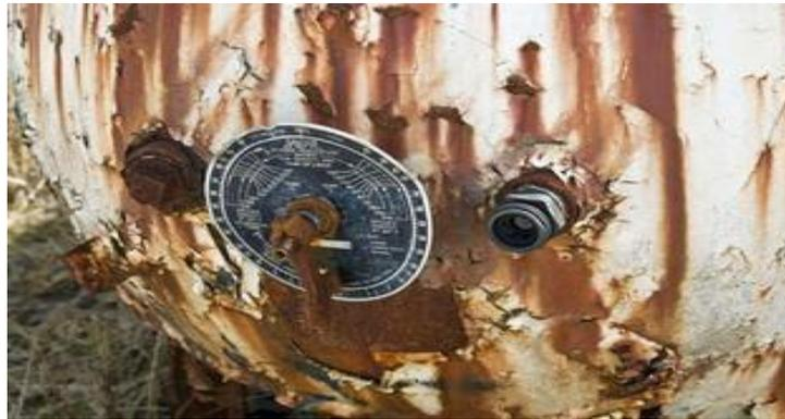
Figure. 1. Condition of a Corroded Pressure Vessel.
