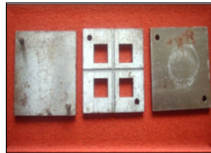
Fig.1 Standard mould for fabrication of heat cure acrylic samples.
