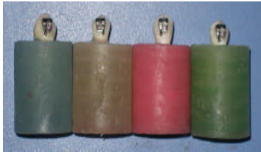
Fig. 1. Brackets bonded to teeth mounted in acrylic blocks. Acrylic blocks color coded to differentiate the four reconditioning groups.
