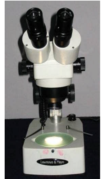
Fig. 3. Lawrence and Mayo Stereomicroscope used to evaluate the adhesive remaining on the tooth
