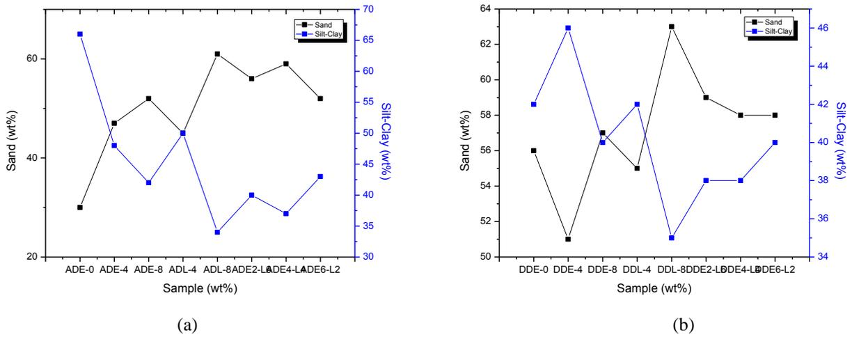
Figure 6a-b Sieve and Grading test analysis of DD and AD with eggshell and lime composition
