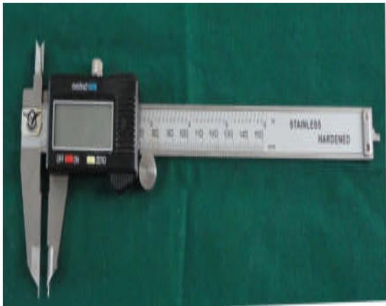
Fig. 5. Calibrated digital vernier caliper with modified tips
