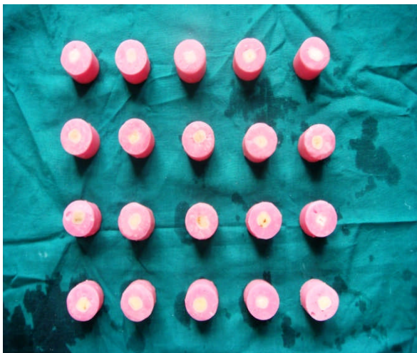
Fig.2 Tooth Specimens mounted on selfcure resin
